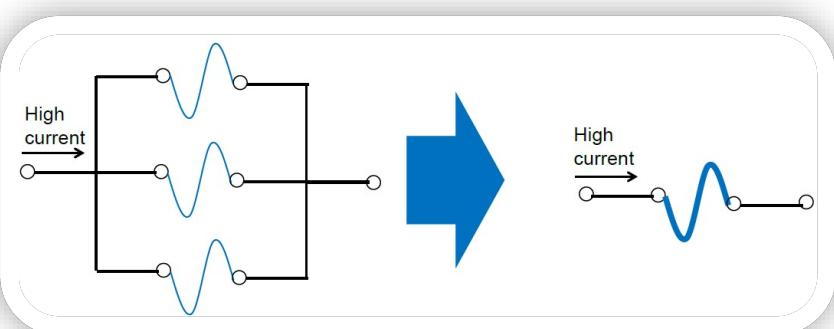
The CMF high power surface mount fuses build on AEM advanced manufacturing technology. The solid, robust structure assures reliable operation in environments where temperature cycling and high mechanical vibration are present. The devices singular fuse link/terminal construction eliminates problems that occur with traditional ceramic tube interconnection techniques
