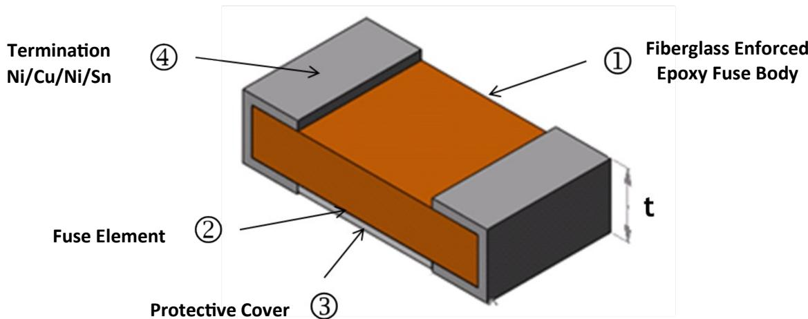
With patent technology and by integrating the advanced think film technology, AEM thin film fuses offer a fusing characteristic from very fast acting to high in-rush current. The fiberglass enforced epoxy fuse body and bi-metal fuse element make fuse to provide protection at low fusing temperature.
