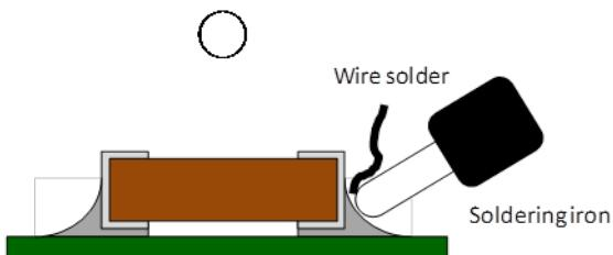
Fig 3 Correct handling method of soldering iron
