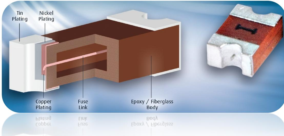
One of the industry's smallest 250V surface mount fuses, the AirMatrix product series are primarily designed for overcurrent protection of line voltage circuits and are widely used in power, battery and server applications. The innovations of AEM's unique material, product design and manufacturing processes provide better reliability, stability and performance.
