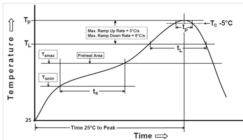
\* Recommended Temperature Profile for Wave Soldering
