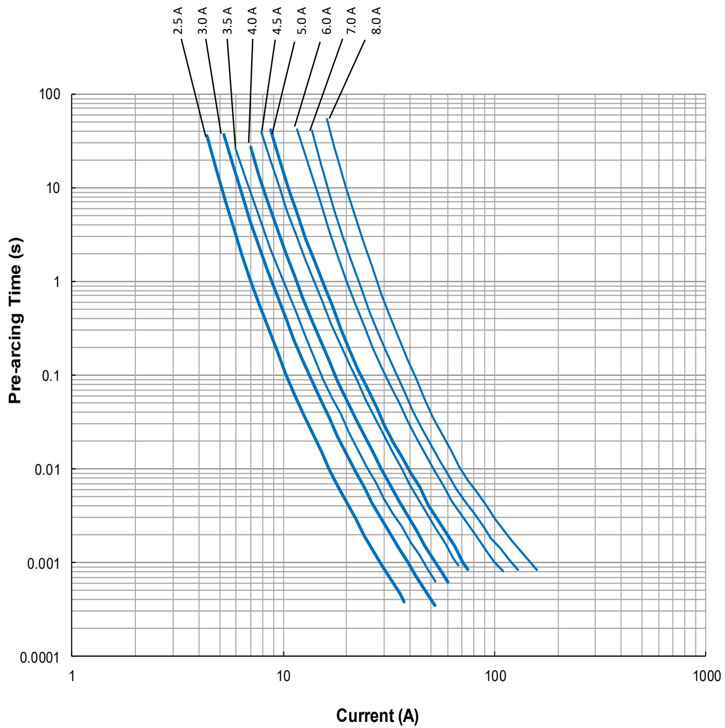
**SolidMatrix® Surface Mount Fuses****VH Series (Voltage High), 1206 Size****Average  $I^2t$  vs. t Curves:**
