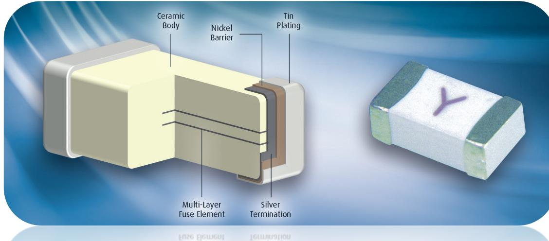
Fuse links and arc suppressing material are buried inside of fuse body. When fuse link opens, there is no fly arc or spark leak. Multiple fuse links design in parallel could improve the amperage rating and save board space. Fuse element diffused into ceramic body, so the integrity of fuse body is maintained and the airtight package is preserved.
