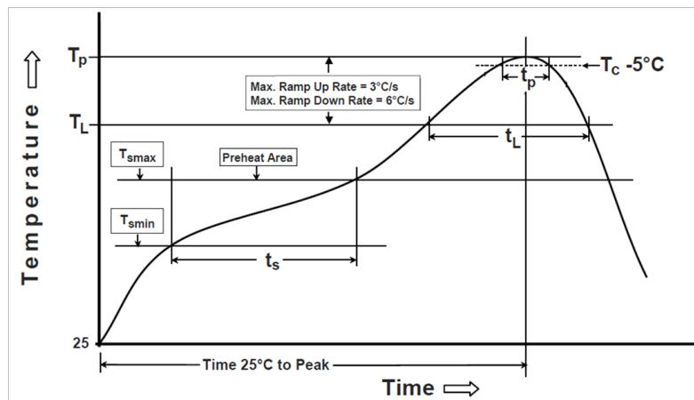
\* Recommended Temperature Profile for Wave Soldering
