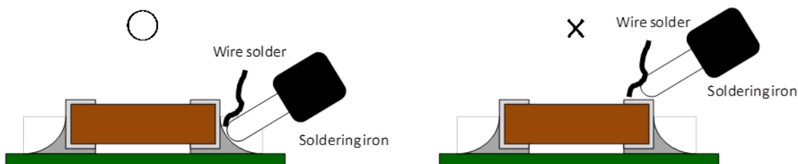
Fig 3 Correct handling method of soldering iron
